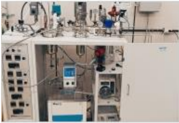
Super critical high pressure Equipment
